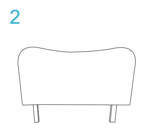
Attach 2 x legs (B) to 1 x bedhead (A) as shown and secure with 6 x washers (C) and 6 x bolts (D). Tighten with an Allen Key (E).
